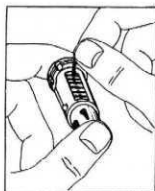
Fig. 69—Inserting Tumbler Springs
