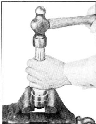
Fig. 13—Installing Mainshaft Bearing Cup
