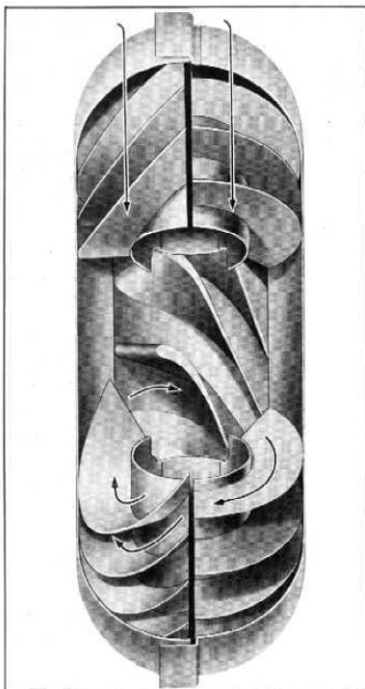
Fig. 155—Oil Flow Through Converter
