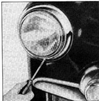
Fig. 60—Removing Headlamp Rim
