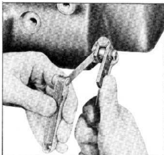
Fig. 129—Checking Clearance Between Parking Lock Lever and Steel Washer
