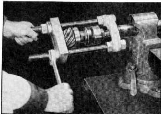
Fig. 12—Pressing Pinion into Propeller Shaft Coupling
