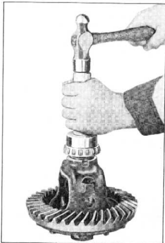
Fig. 14—Replacing Differential Bearing
