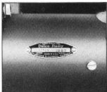
Generator serial and model number are located on a metal plate staked on the generator body just forward of armature terminal (fig. 2).
