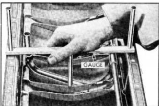
Fig. 26—Checking Oil Trough Depth
