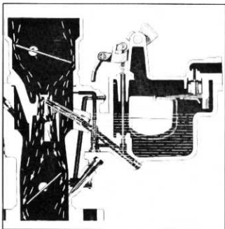
Fig. 80—Carburetor Operation When Starting Engine
