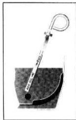
Fig. 2—Oil Gauge Rod
