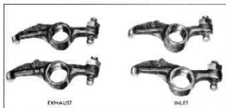
Fig. 18—Valve Rocker Arm Identification
