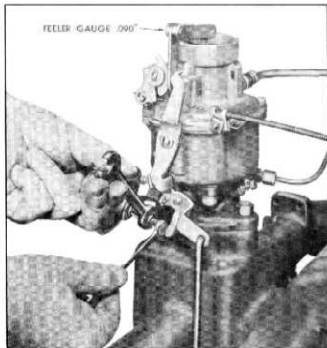
Fig. 98—Throttle Return Check Adjustment
