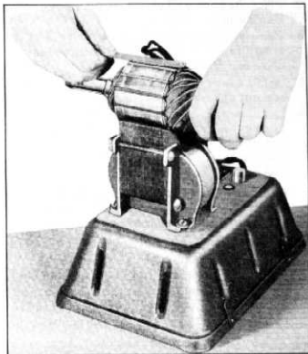
Fig. 33—Armature Test for Short
