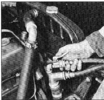
Fig. 121—Reverse Flushing Radiator
