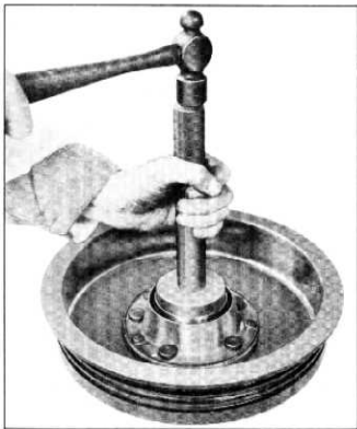
Fig. 12—Installing Bearing Cup
