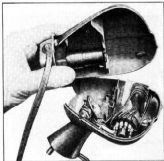
Fig. 68—Installing Test Lamp
