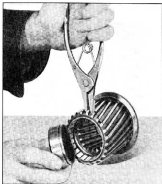
Fig. 13—Removing Synchronizer Ring
