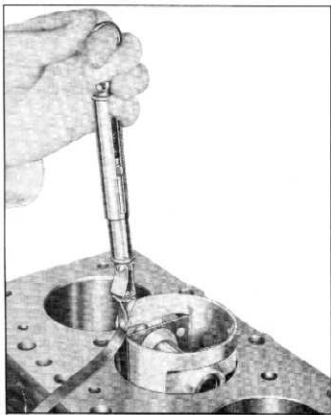
Fig. 46—Fitting Aluminum Pistons
