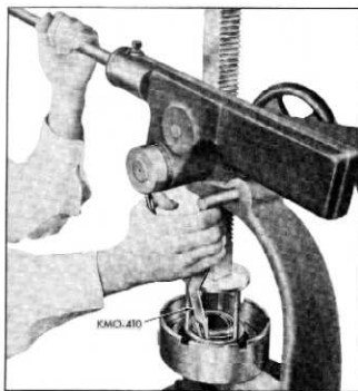
Fig. 90—Remove Clutch Spring Snap Ring
