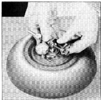
Fig. 89—Check End Play of Turbine Bolt
