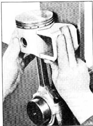
Fig. 65—Checking Piston and Connecting Rod Assembly
