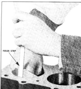
Fig. 45—Fitting Cast Iron Pistons
