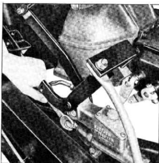
Fig. 9—Adjusting Toe Board Clearance
