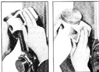
Fig. 66—Checking Piston and Connecting Rod Assembly for Twisted Connecting Rod
