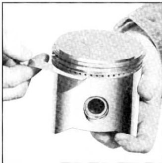
Fig. 68—Checking Piston Ring Clearance in Ring Groove
