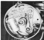
Ignition distributor serial and model number are located on the distributor breaker plate which is under distributor cap (fig. 3).
