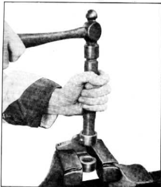
Fig. 8—Removing Pivot Shaft Bushings
