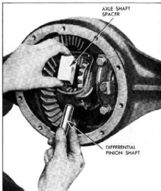
Fig. 3—Removing Axle Shaft Spacer
