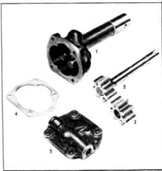
Fig. 24—Layout of Oil Pump Parts
