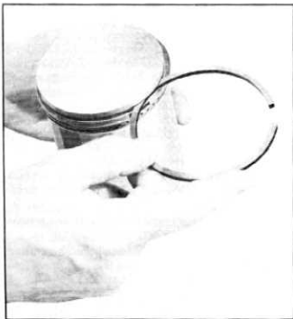
Fig. 67—Rolling Piston Ring in Ring Groove
