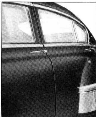
Fig. 42—Door Too Far "Out" at Pillar
